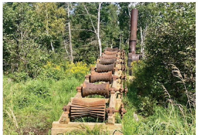
Below left to right: Lead volunteer, Roger Morneault, standing next to the first phase of the Tramway Reconstruction Project. Modified version of the tramway log discharge roller ramp.
