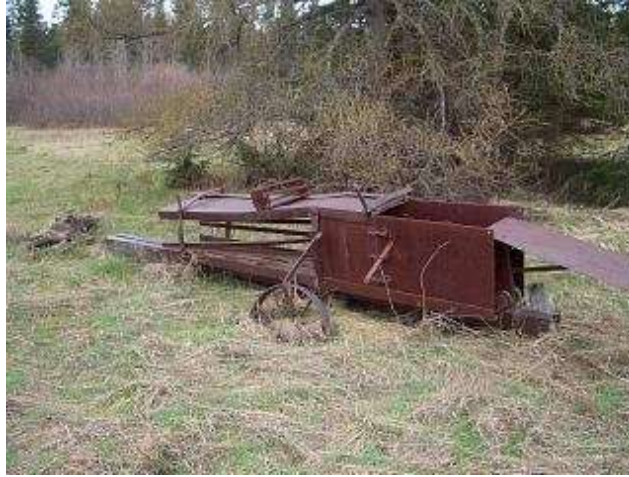
Hay baler at Seven Islands. Horses walked in a circle around the baler connected to turnstyle piston which compressed hay into bales. Bales were easier to store and transport than loose hay. (Cassie Vaillancourt photo)
